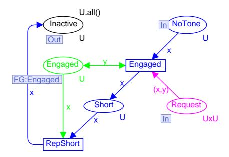
Next, let us consider how the *Breaking of a connection by the Sender* is performed, i.e., the page *BreakSen*. This page has only one additional state for the telephones:
